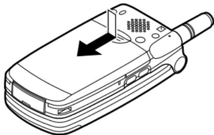
2. Slide the SIM card into the SIM holder.
