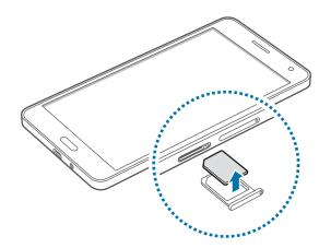
4 Insert the SIM card tray back into the SIM card tray slot.
