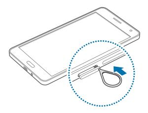
Ensure that the ejection pin is perpendicular to the hole. Otherwise, the device may be damaged.
