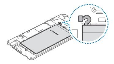
6 Push the back of the battery with your fingers and remove the battery.
