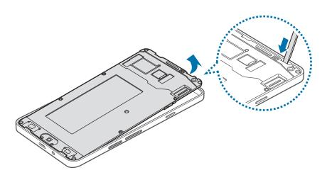
5 Disconnect the battery connector as shown in the image below.
