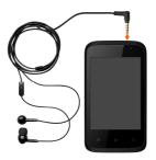
You will be required to plug in your headset before starting the FM Radio. The headset works as antenna for the FM radio.
