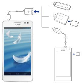
To connect your phone to another phone, make sure that the phone you wish to connect to supports the USB mass storage function and has a microSD card installed. To establish the connection and read data stored on the microSD card:
