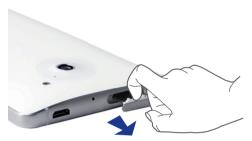
3. Follow the directions on the micro-SIM card tray to place the micro-SIM card in the tray, and then replace the tray.
