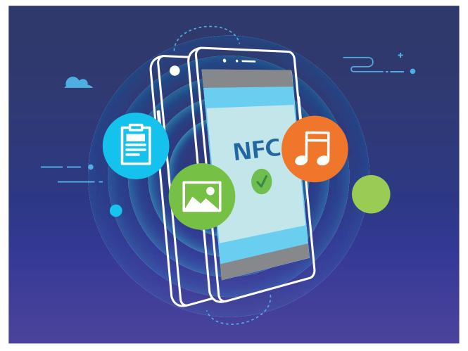
**Use NFC to send data**: Open Settings, then touch **Device connectivity** and enable **NFC** and **Huawei Beam**. Select the files to be sent and touch **Share** > **Huawei Beam**. Keep your Phone unlocked and the screen on. Place the NFC detection areas of both devices close together. Once a connection is established, the transmitting device will play an audio prompt and the sharing screen will minimise. Touch the transmitting device's screen to begin sending files.
