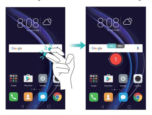
• Press the volume up and power buttons simultaneously and select the desired recording mode.
