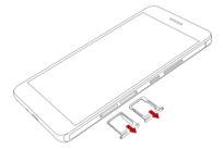
**3.** Place the micro-SIM and nano-SIM cards into their respective card trays. Make sure the gold contact areas and bevelled edges of the cards are facing the right directions (a). Then push the card trays back into place (b).
