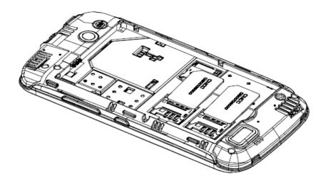
3. Finally insert the battery and replace the rear cover of the mobile phone.
