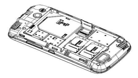
3. Finally insert the battery and the rear cover of the mobile phone.
