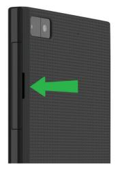
2. With the metal contacts facing you, insert the micro SIM card into the bottom slot.
