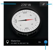
Interference indicator. Move your device away from metal, then rotate and tilt your device until the indicator disappears.
