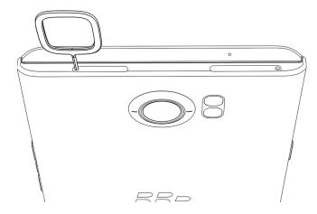
4. Pull out the tray completely and remove the media card.
