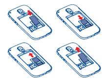
Inserting or removing the SD card
