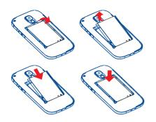
Insert and click the battery into place, then close the telephone cover.
