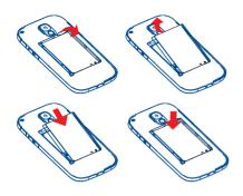
Insert and click the battery into place, then close the telephone cover.
