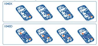
Place the SIM card with the chip facing downwards and slide it into its housing. Make sure that it is correctly inserted. To remove the card, press it and slide it out.
