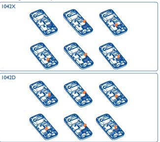
To release the microSD card holder, slide it in the direction of the arrow and lift it. Then insert the microSD card with the golden contact downward. Finally, turn down the microSD holder and slide it in the opposite direction to lock it.
