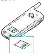
6. Place the battery back on the phone. Slide the battery up towards the catch until it locks into place. Make sure that the battery is properly installed before switching on the power.
